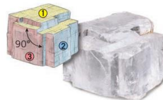
D. Cleavage in three directions at 90° angles. Example: Halite
