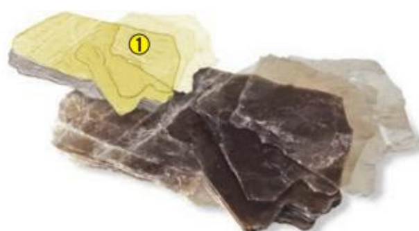
A. Cleavage in one direction. Example: Muscovite
