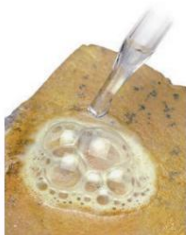
▲ SmartFigure 1.21 Calcite reacting to dilute hydrochloric acid. (Photo by Chip Clark/Fundamental Photographs)
