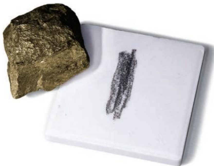
▲ SmartFigure 1.6 Using streak to help identify a mineral.
