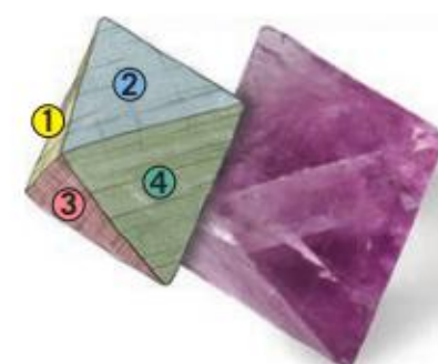
F. Cleavage in four directions. Example: Fluorite
