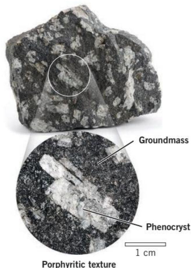
▲ Figure 2.5 The large crystals in a porphyritic rock are called phenocrysts , and the matrix of smaller crystals is called groundmass .
