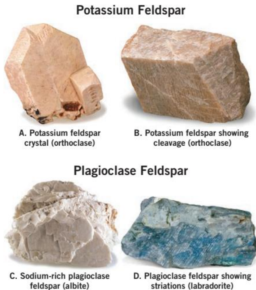
▲ Figure 1.25 Feldspar group. A. Characteristic crystal form of potassium feldspar. B. Like this sample, most pink feldspar belongs to the potassium feldspar subgroup. C. Most sodium-rich plagioclase feldspar is light colored and has a porcelain luster. D. Calcium-rich plagioclase feldspar tends to be gray, blue-gray, or black in color. Labradorite, the variety shown here, exhibits striations.
