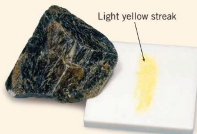
► Figure 1.9 Using streak to assist in describing luster.
