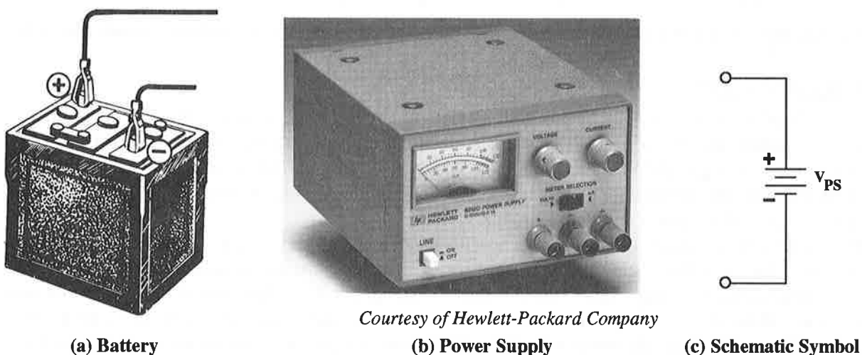
FIGURE 1-2: Commonly used voltage sources and the schematic symbol for dc voltage sources.
