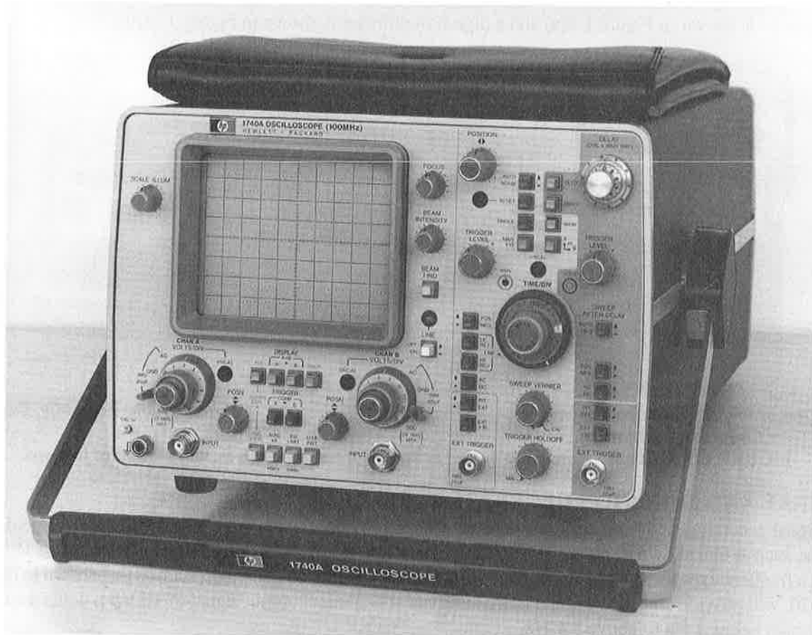
FIGURE 1-8: Oscilloscopes provide a visual measurement of dc voltage and ac signal voltage.
