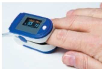
FIGURE 5-17 ■ Pulse oximeter. This device is used in ambulances and other healthcare settings to provide a quick measurement of the percentage of the patient's hemoglobin that is saturated with oxygen ( \%\text{SpO}_2 ) and the pulse rate (PR) in beats per minute (bpm). Both of this patient's measurements are within normal limits. Note: A pulse oximeter may not provide an entirely accurate measurement of the \%\text{SpO}_2 in patients with darker skin.
