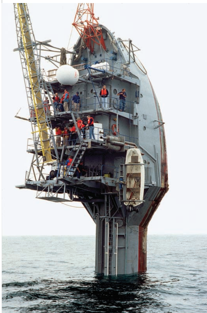
FIGURE 1.11 R/V FLIP , short for floating instrument platform , operated by Scripps Institution of Oceanography, provides a stable platform for research at sea. (a) Most of the hull consists of a hollow tube that floats while the vessel is towed into position. When the hull is flooded and sinks, FLIP swings into a vertical position (b) in which it is largely unaffected by the rise and fall of waves.
