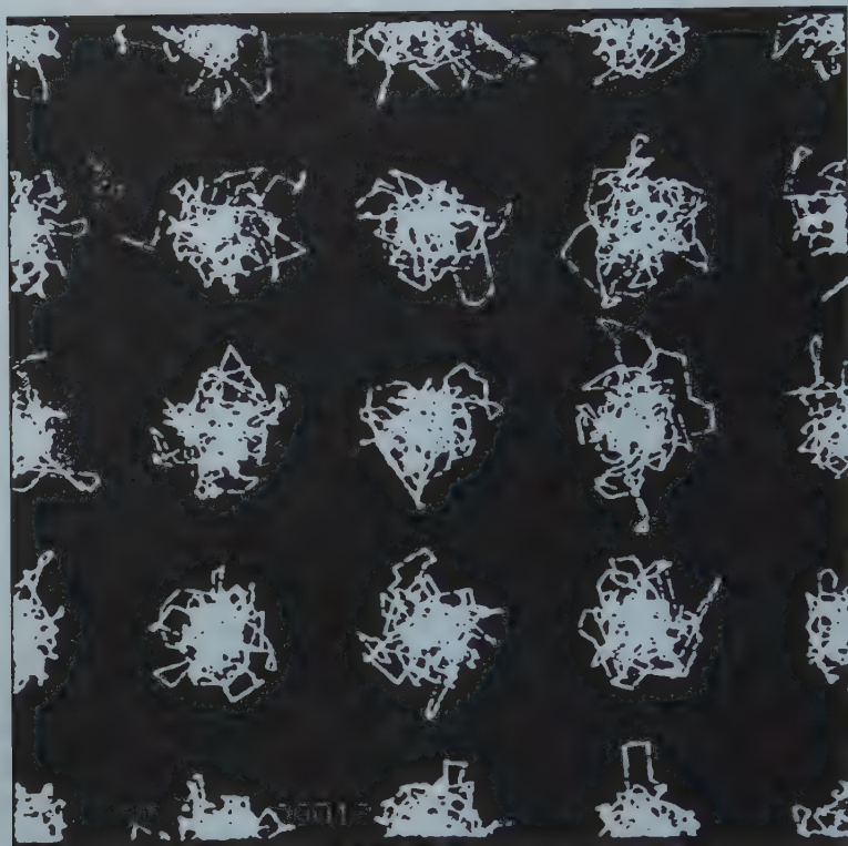
FIGURE 1.2-1 Plots of the theoretical pathlines of atoms in a crystal. (Calculated by Alder, B.J., and Wainwright, T., J. Chem. Phys. , 31(2), 459–466, 1959, and reprinted with permission.)
